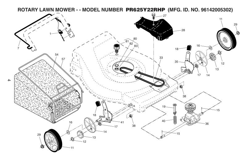
ROTARY LAWN MOWER - - MODEL NUMBER PR625Y22RHP (MFG. ID. NO. 96142005302)
