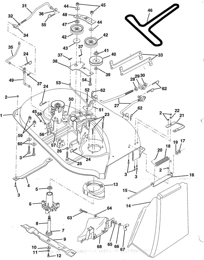
12.5 HP 38" TRACTOR-MODEL NO. LR125 (HU125R38MA), PRODUCT NO. 954 00 05-22 **MOWER DECK**
