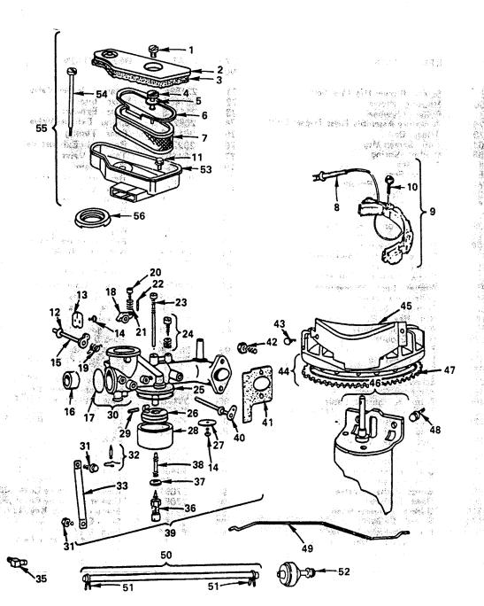
The same of the same of the same ROPER LAWN TRACTOR-MODEL NUMBER LT110ER ENGINE BRIGGS AND STRATTON-MODEL NUMBER 253707, TYPE NUMBER 0154-01 **CARBURETOR**
