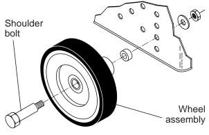
MODELS WITH "QUICK ADJUST" WHEEL HEIGHT ADJUSTERS **NOTE**: For shipping purposes, the rear wheels on your lawn mower may not be adjusted to the same position as the front wheels. Before operating mower adjust all wheels to the same cutting height.
