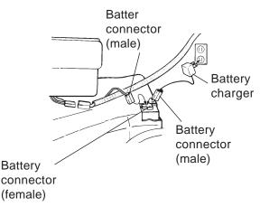
**ACAUTION:** Always disconnect the engine connector (male) from the battery connector (female) to prevent accidental starting when transporting or storing your lawn mower after the season.
