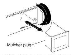
MULCHER PLUG BUILT INTO REAR DOOR
