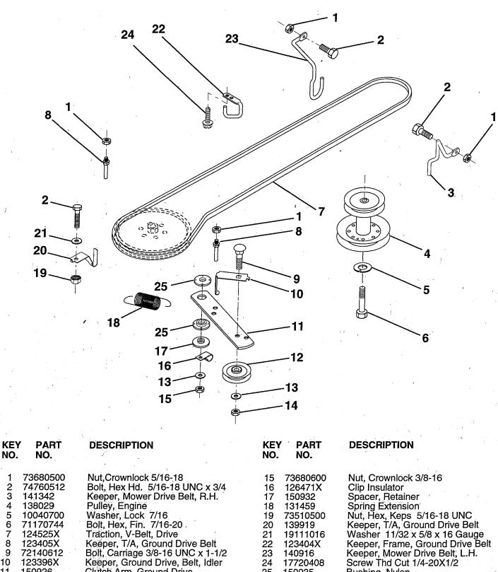
NOTE: All component dimensions given in U.S. inches. Washer 13/32 x 13/16 x 16 Ga. 1 inch = 25.4 mm Nut, Centerlock 3/8-16 UNC
