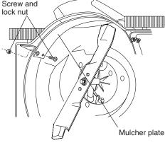
Some models have a seperate mulcher plug, other models have the mulcher plug built into the rear door. To convert to bagging or discharging, the plate or plug (if so equipped) must be removed from the discharge opening of the lawn mower.
