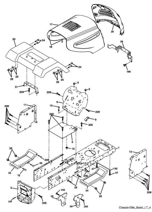
TRACTOR - - MODEL NUMBER MC1136 (MC1136B), PRODUCT NO. 964 77 30-01 CHASSIS AND ENCLOSURES
