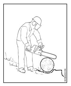
Bucking is cutting a log into sections.
