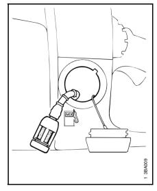
STIHL recommends the use of a suitable tool (e.g. screwdriver end of combination wrench) to tighten the cap securely.
