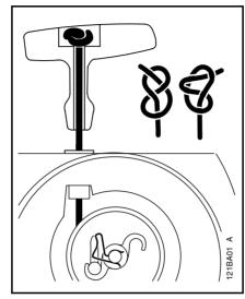
Remove remaining rope from rotor - thread the new rope - 3.5 mm (0.14") dia. and 960 mm (37.8") long - into the rotor and secure it with a simple overhand knot. Thread other end - from inside - through the rope guide bush and through the of starter grip and secure with special knot - do not wind rope onto rotor.
