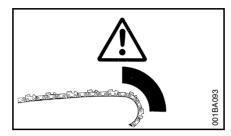
powerful force used to cut wood can be reversed (and work against the operator). If the rotating chain is suddenly stopped by contact with any solid object like a log or branch or is pinched, the reactive forces may occur instantly. These reactive forces may result in loss of control which may, in turn, cause serious or fatal injury. An understanding of the causes of these reactive forces may helpyou avoid loss of control.
