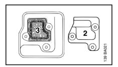
If the engine is low on power, check the spark arresting screen inside the muffler. Take out the nuts (1). Remove the cover (2). Remove the spark arresting screen (3).
