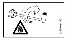
Before fueling, clean the filler cap and the area around it to ensure that no dirt falls into the tank.
