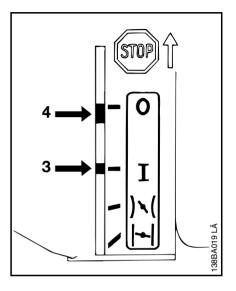
In the "Warm Start" position, continue cranking after engine begins to fire. As soon as the engine runs, **immediately** blip the throttle trigger so that the Master Control lever moves to "Run" -
