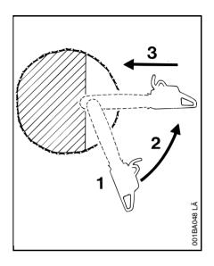
Avoid repositioning the saw more than necessary. When repositioning for the next cut, keep the guide bar fully engaged in the kerf to keep the felling cut straight. If the saw begins to pinch, insert a wedge to open the cut. On the last cut, do not cut the hinge.
