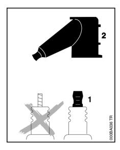
Fit a new spark plug after approx. 100 operating hours or earlier if the electrodes are badly eroded.
