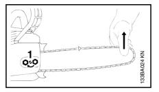
Retensioning during cutting work:
