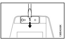
Refit the filter and carburetor box cover and secure it with the twist lock: Heated air is now drawn in from around the cylinder and mixed with cold air this prevents carburetor icing.
