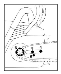
Fit the guide bar over the studs (4) cutting edges on top of bar must point to right and engage the peg of the tensioner slide in locating hole (5) place the chain over sprocket (6) at the same time -
