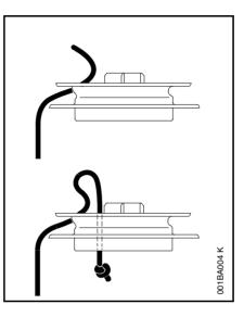
Thread the rope through the rotor and secure it with a simple overhand knot.
