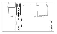
Pry the shutter (1) out of the carburator box cover (summer position) and slide it into the slot (2) (winter position)
