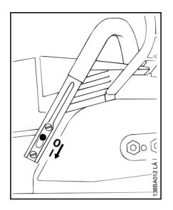
Switching on electric handle heating\*
