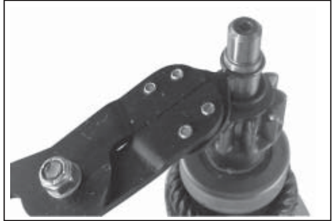
Figure 8-54. Removing Retaining Ring.
