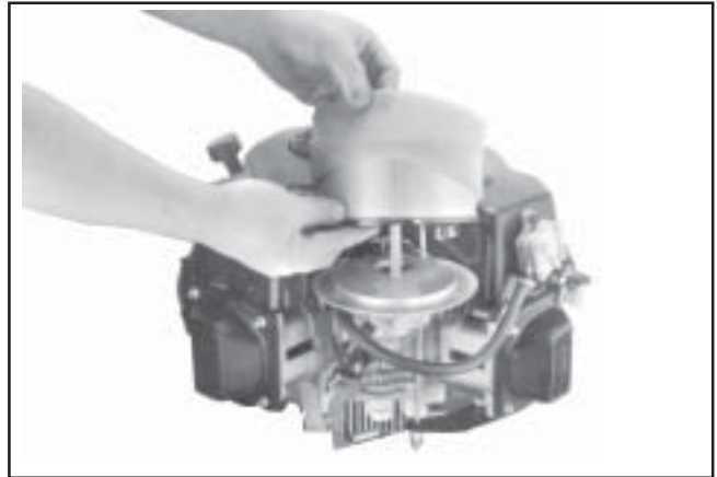
Figure 9-8. Removing Commercial Mower Element and Precleaner.
