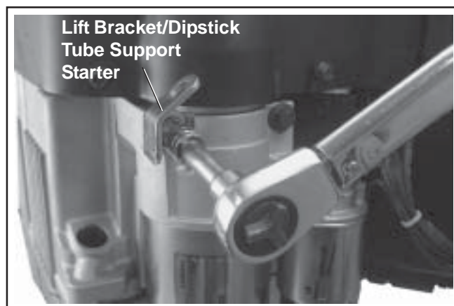
Figure 11-79. Installing Starter and Lift Bracket.
