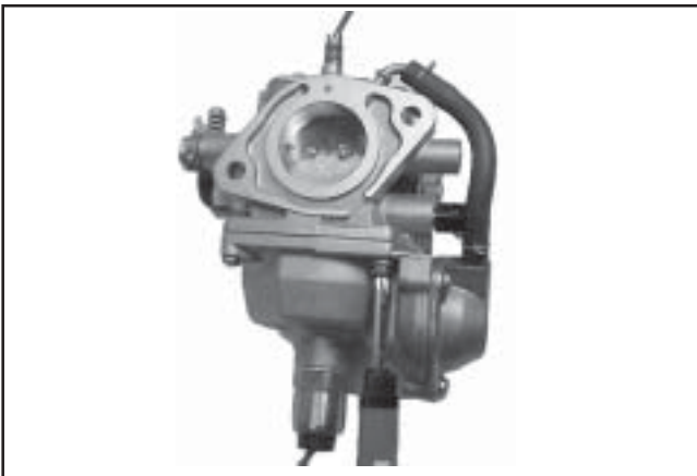
Figure 5-27. Installing Fuel Bowl.
