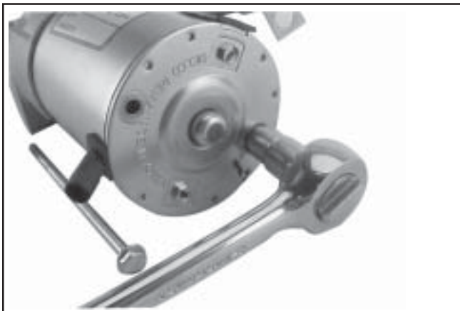
Figure 8-48. Removing Thru Bolts.
