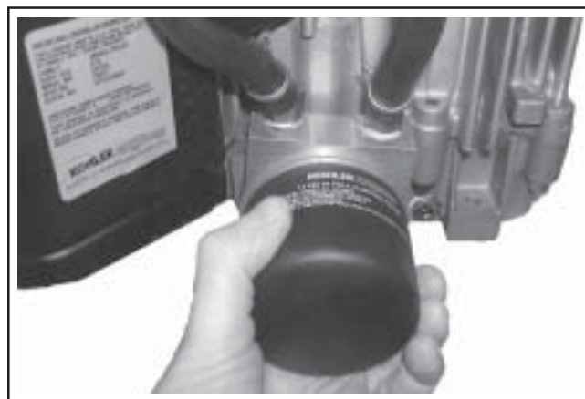
Figure 11-91. Installing and Tightening Oil Filter.
