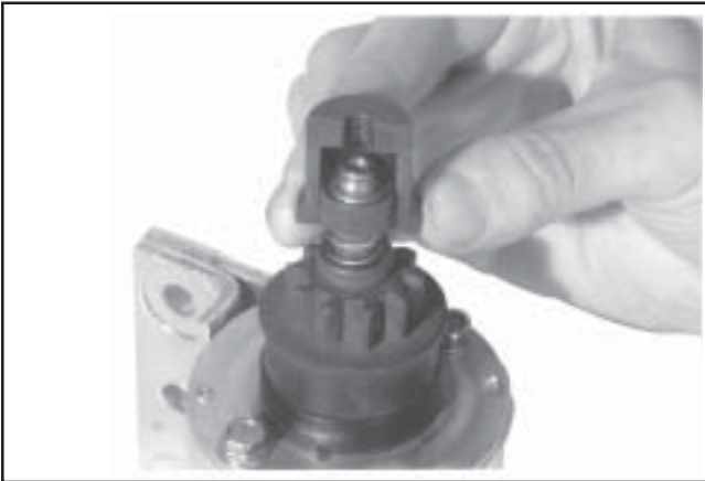
Figure 8-38. Assembling Larger Inner Half Around Spring Retainer.
