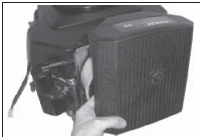
Figure 9-5. Removing Standard Air Cleaner Cover.
