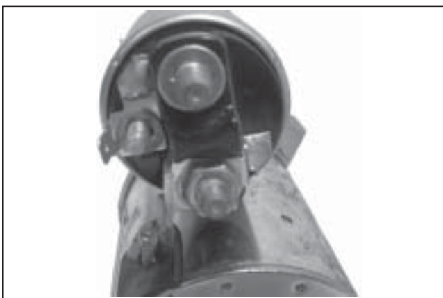
Figure 8-73. Positive (+) Brush Lead Connection.
