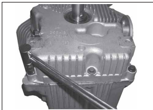
Figure 11-19. Torquing Oil Pan Fasteners.
