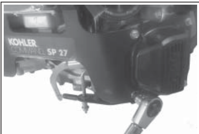
Figure 11-89. Securing Air Cleaner Mounting Bracket.
