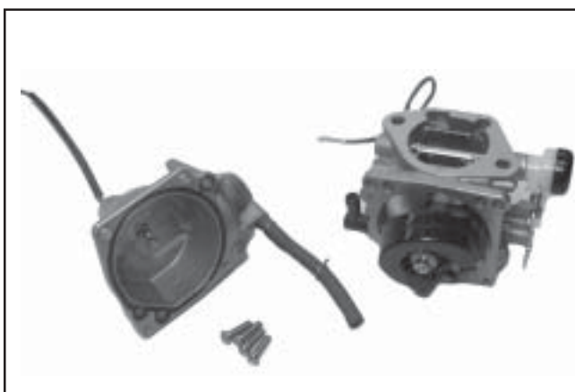
Figure 5-17. Fuel Bowl Removed from Carburetor.
