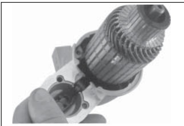
Figure 8-63. Installing Armature and Pivot Lever.
