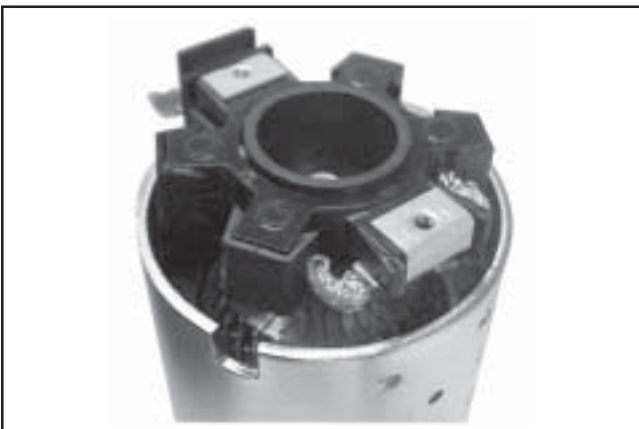
Figure 8-67. Installing Brush Holder Assembly with Supplied Tube.
