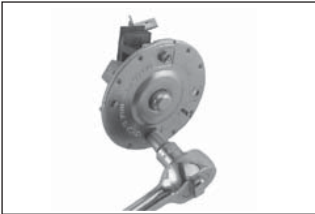
Figure 8-59. Removing Brush Holder.
