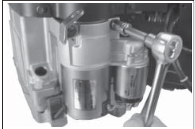
Figure 9-25. Removing Electric Starter Motor.
