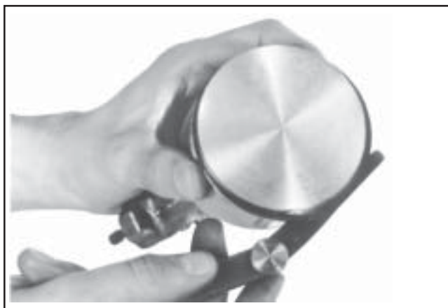
Figure 10-10. Measuring Piston Ring Side Clearance.
