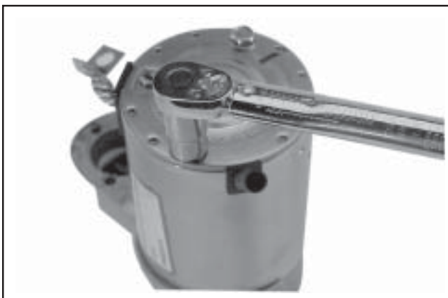
Figure 8-71. Torquing Thru Bolts.
