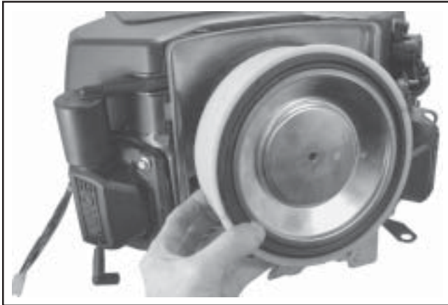
Figure 9-6. Removing Standard Element and Precleaner.
