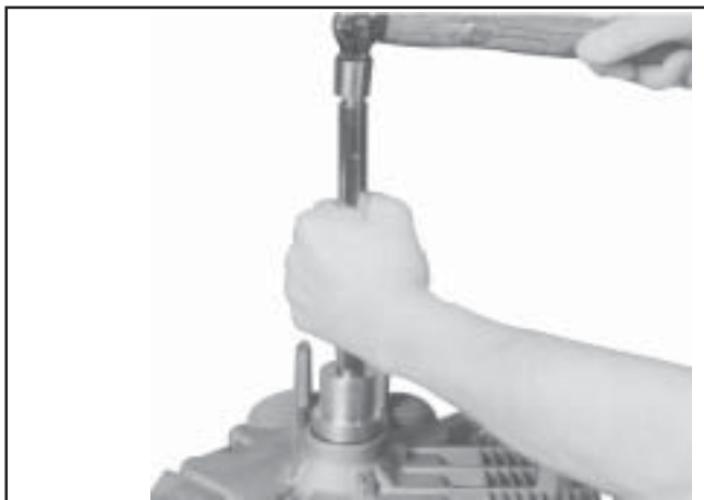
Figure 11-2. Installing Oil Seal in Crankcase.
