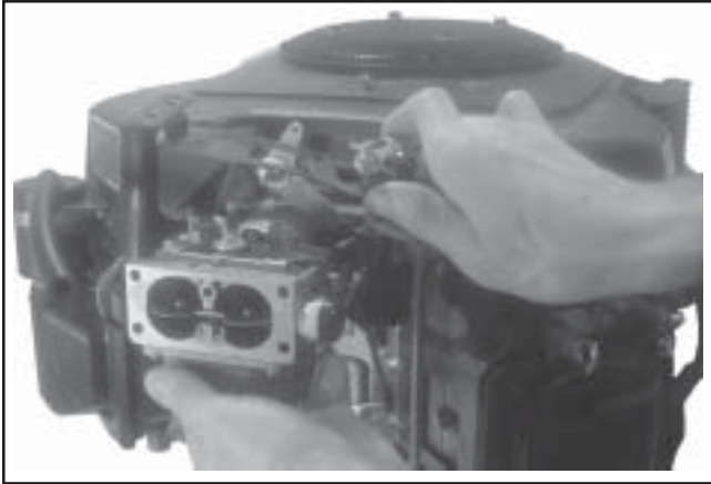
Figure 9-22. Removing Carburetor and Linkage (Two-Barrel Model Pictured).
