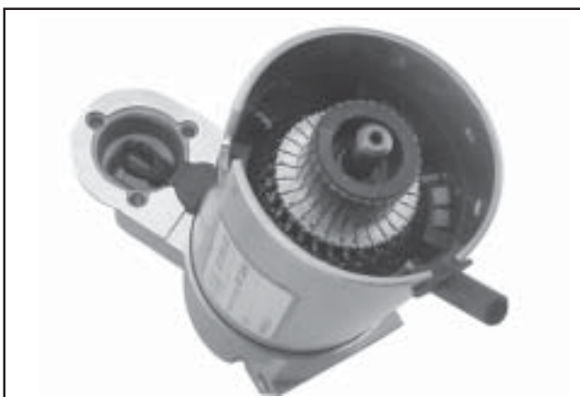
Figure 8-65. Installing Frame and Drain Tube.
