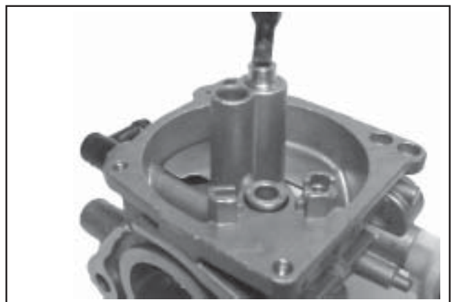
Figure 5-20. Installing Main Nozzle and Main Jet.
