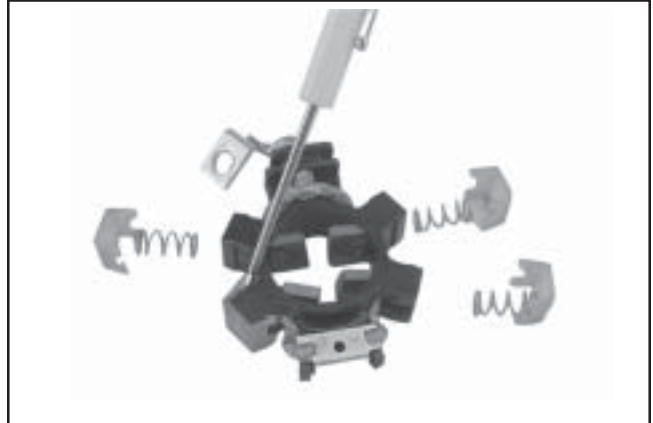
Figure 8-68. Removing Retaining Clips.
