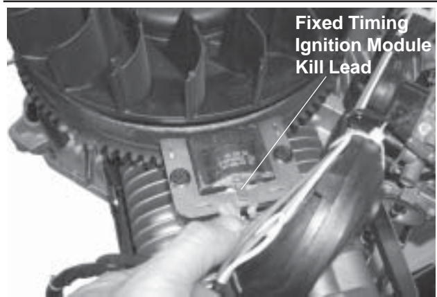
Figure 9-38. Disconnect Lead(s) from Ignition Modules.
