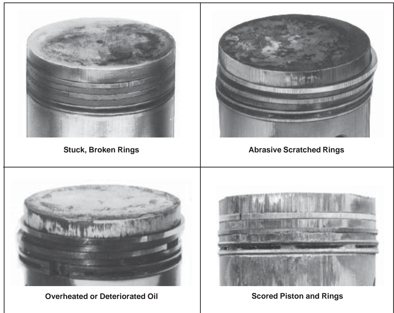
Figure 10-8. Common Types of Piston Damage.
