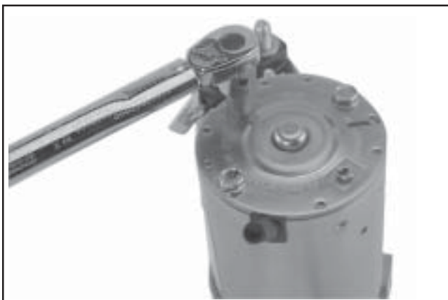
Figure 8-72. Torquing Brush Holder Screws.
