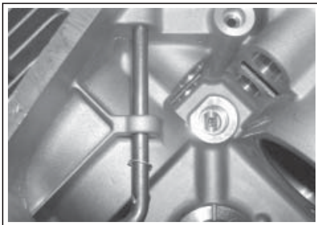
Figure 11-5. Installing 8 mm Governor Cross Shaft.
