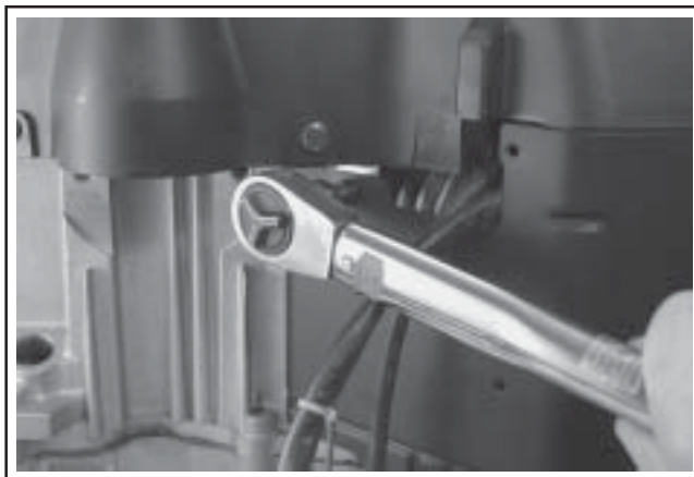
Figure 11-61. Tightening Short Screws for Outer Baffles.
