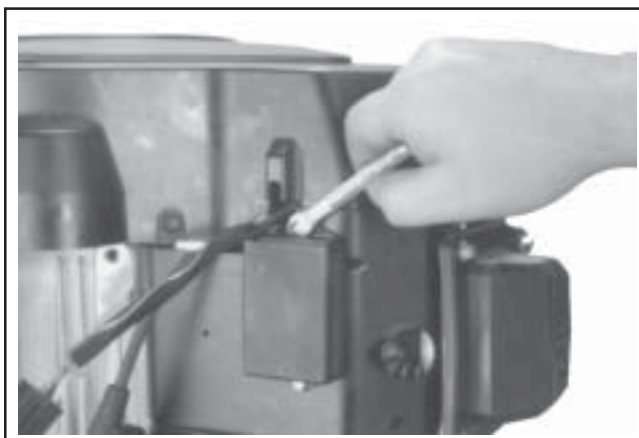
Figure 9-27. Loosening Spark Advance Module (Applicable Models).
