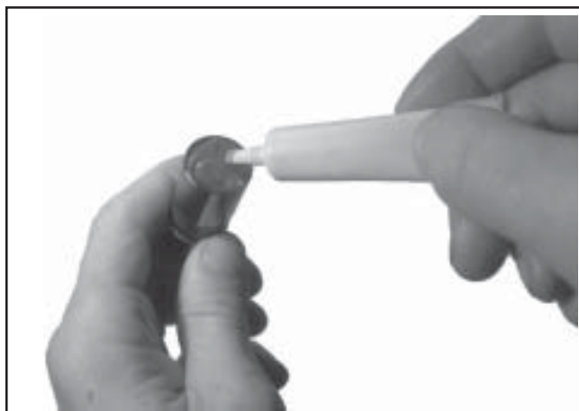
Figure 11-30. Applying Camshaft Lubricant to Bottom of Lifters.
