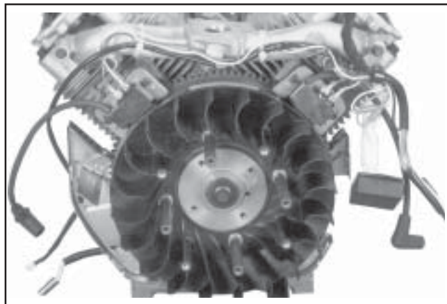
Figure 8-6. Capacitive Discharge Ignition System with Spark Advance.
