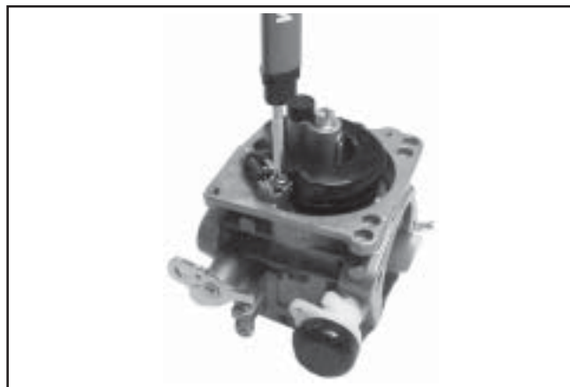
Figure 5-24. Installing Float Assembly.
