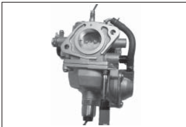
Figure 5-16. Installing Fuel Bowl.
