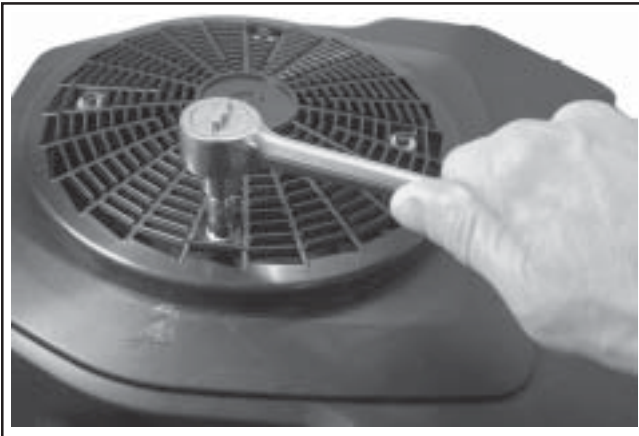
Figure 9-30. Removing Flywheel Screen.
