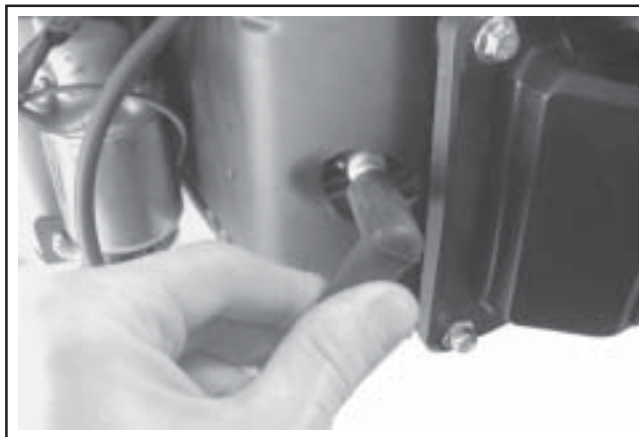
Figure 11-93. Connect Spark Plug Leads.
