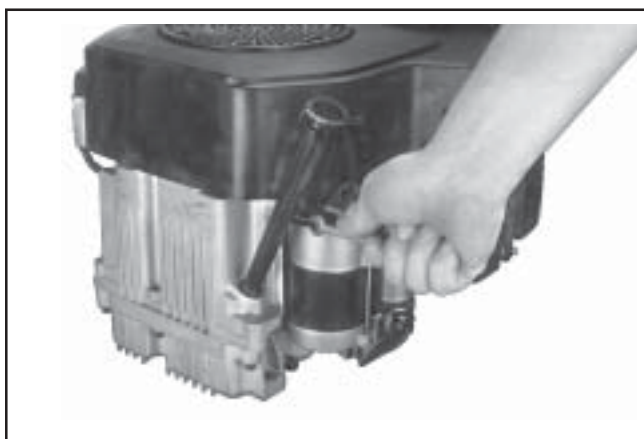
Figure 9-3. Removing Oil Fill Tube Bracket.
