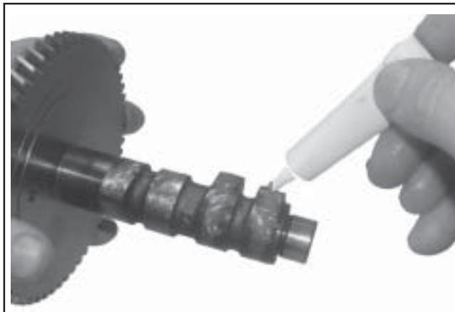
Figure 11-12. Apply Camshaft Lubricant to Cam Lobes.
