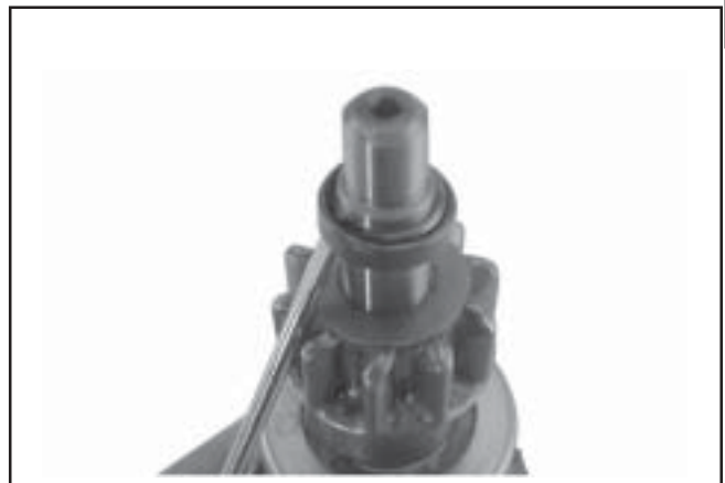
Figure 8-61. Installing Stop Collar and Retainer.
