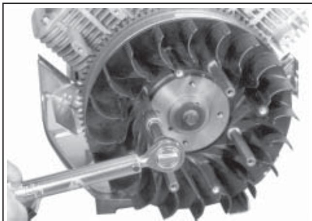
Figure 11-29. Torquing Supports for Metal Screen (Some Models).
