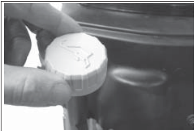
Figure 9-2. Removing Oil Fill Cap/Dipstick.
