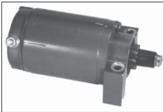
Figure 8-41. Starter Assembly Match Marks.
