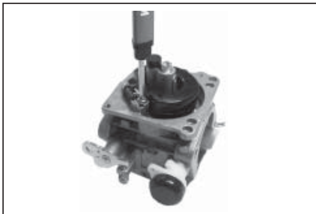
Figure 5-14. Installing Float Assembly.
