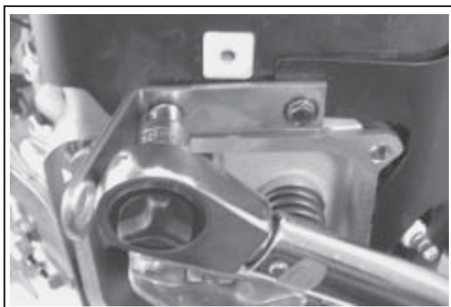
Figure 11-60. Tightening Outer Baffle Front Screws.
