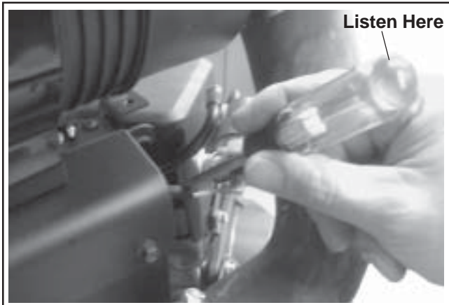
Figure 5B-17. Checking Injectors.
