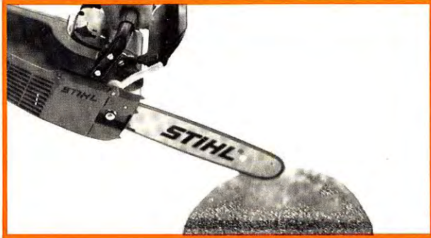
Checking chain lubrication
