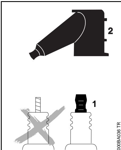
**⚠** To reduce the risk of fire and burn injury, use only spark plugs authorized by STIHL. Always press spark plug boot (2) snugly onto spark plug terminal (1) of the proper size. (Note: If terminal has detachable SAE adapter nut, it must be attached.) A loose connection between spark plug boot and ignition wire connector in the boot may create arcing that could ignite combustible fumes and cause a fire.
