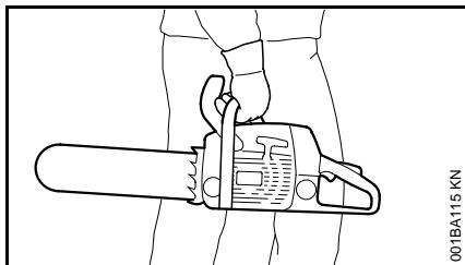
It may be carried only in a horizontal position. Grip the front handle in a manner that the machine is balanced horizontally. Keep the hot muffler away from your body and the cutting attachment behind you.
