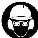
Wear an approved safety hard hat to reduce the risk of injury to your head. Chainsaw noise may damage your hearing. Wear sound barriers (ear plugs or ear mufflers) to help protect your hearing. Continual and regular users should have their hearing checked regularly.
