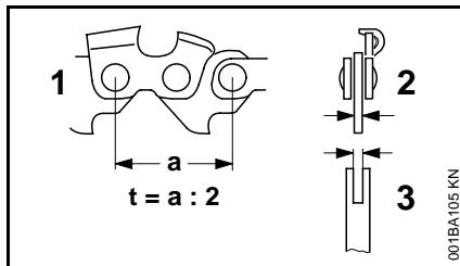
You can run chains of different pitches on this chainsaw – depending on the chain sprocket (see "Specifications"):
