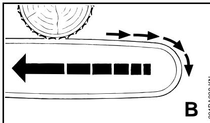
Pushback occurs when the chain on the top of the bar is suddenly stopped when it is pinched, caught or encounters a foreign object in the wood. The reaction of the chain may drive the saw rapidly straight back toward the operator and may cause loss of saw control.
