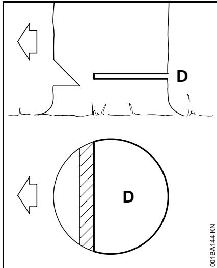
Drive wedges into the felling cut where necessary to control the fall.
