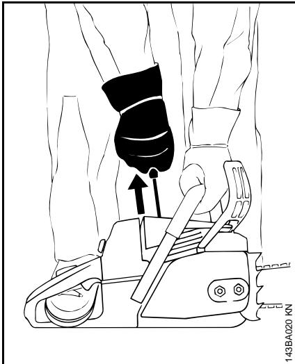
If the engine is new, pull the starter several times to prime the fuel system.
