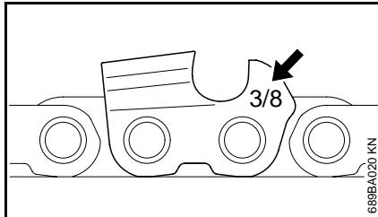
The chain pitch (e.g.  $\frac{3}{8}$ ") is marked on the depth gauge end of each cutter.
