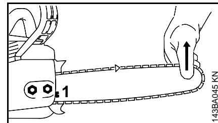
Retensioning during cutting work:
