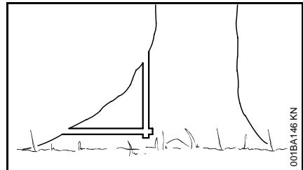
If the tree has large buttress roots, cut into the largest buttress vertically first (horizontally next) and remove the resulting piece.
