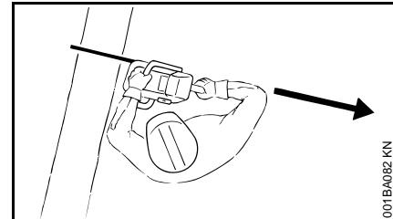
Position the chainsaw in such a way that your body is clear of the cutting attachment whenever the engine is running. Stand to the left of cut while bucking.
