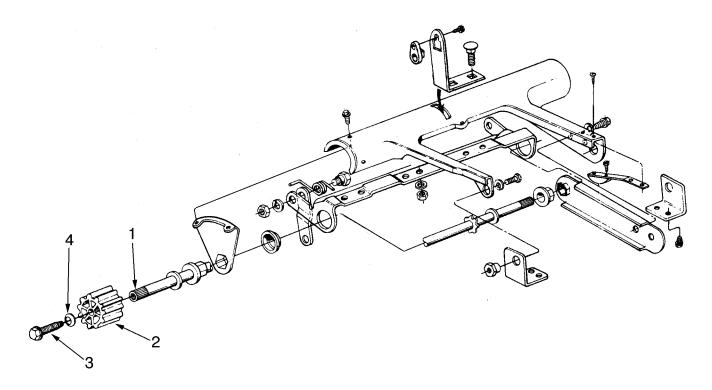
*NOTE:* For Model Series 220 thru 229 it will be necessary to order replacement pinion drive halves. Order 4 each of a part number 717-0623.
